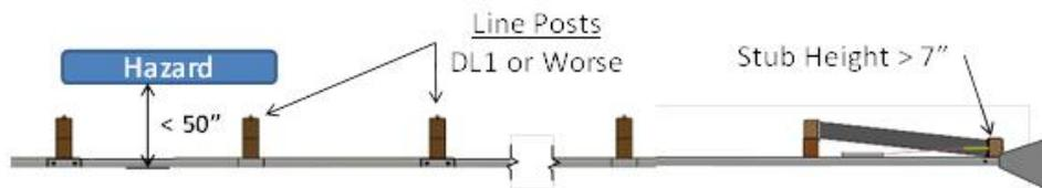
$$\text{Combination Mode} = \left\{ \begin{array}{l} \text{Hazard within } 50'' \text{ behind rail, and} \\ \text{Stub height } > 7'' \text{ and} \\ \text{Line posts DL1 or worse} \end{array} \right\} \text{High}$$
