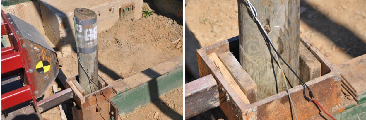
1 2 Figure 5. Rigid steel sleeve used for post mounting.
