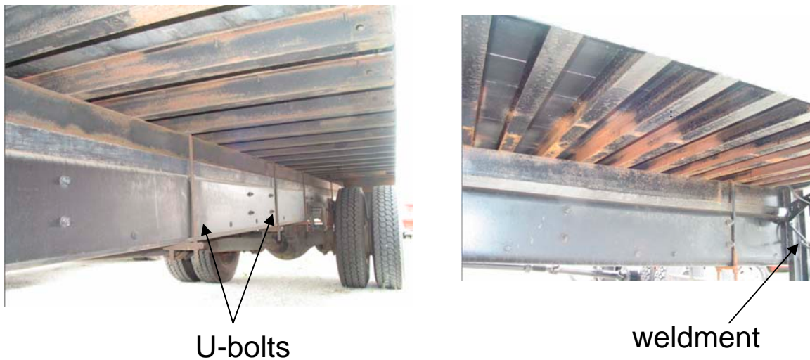
Figure 24 : Bed-frame is connected to main frame-rails of truck with weldments and U-bolts.
