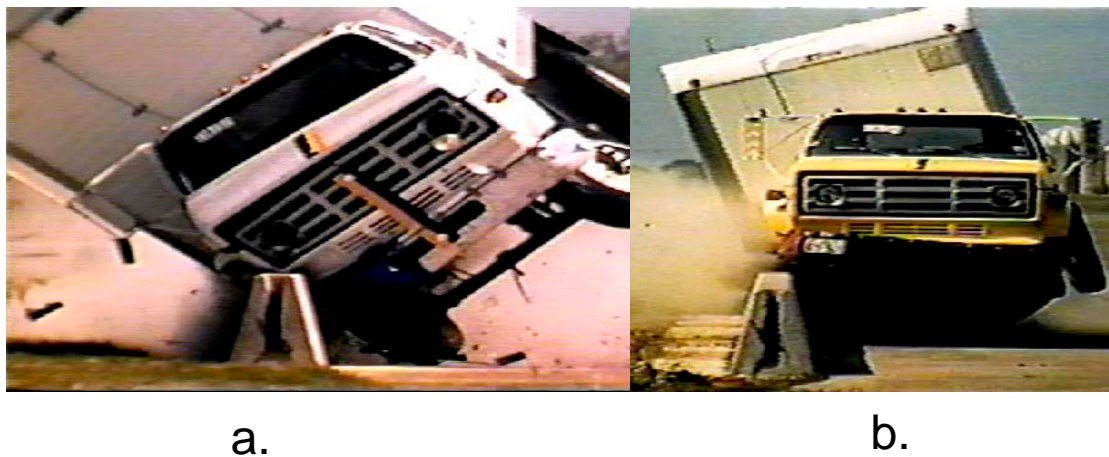
Figure 26: a) Truck-bed “rigidly” restrained (TTI Test 7147-17) and b) Truck-bed translates laterally with respect to truck body due to insufficient lateral constraint (TTI Test 7147-16). 10,11
